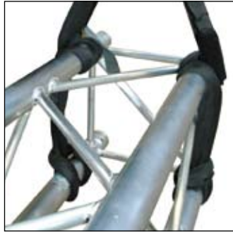
Rectangular truss 2 sling choke extra wrap upper chords outside
