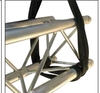
Rectangular truss 1 sling wrap lower chords
