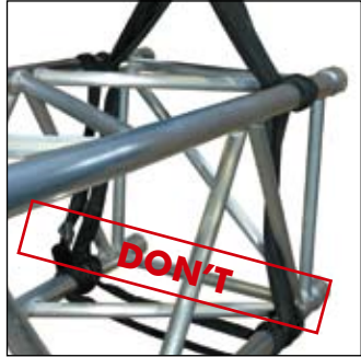
Rectangular truss 1 sling wrap lower/upper chords
