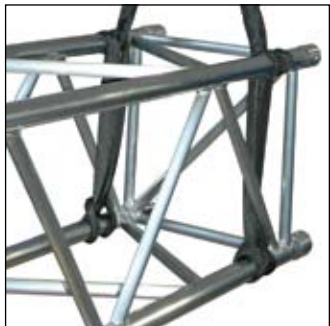
Rectangular truss 2 sling choke lower extra wrap upper chords
