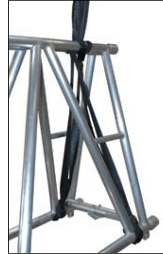
Folding truss 2 sling choke lower chords extra wrap upper chords
