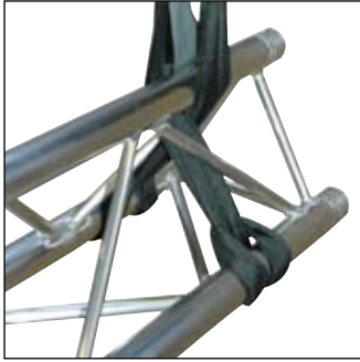
Triangular truss apex up 2 sling choke
