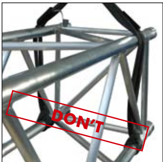
Rectangular truss 2 sling choke lower chords
