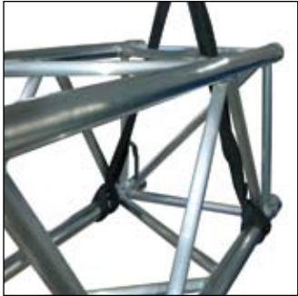
Rectangular truss 2 sling choke lower chords
