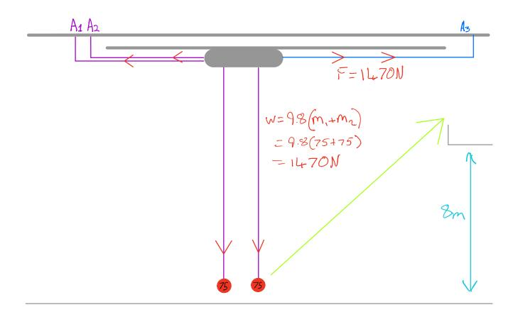
Total force on line A3 is 1470N. The maximum force allowed on line A3 is 1960N, therefore an addition force of 490N is available. The impulse (or acceleration force will need to be equal to or else than 490N)
