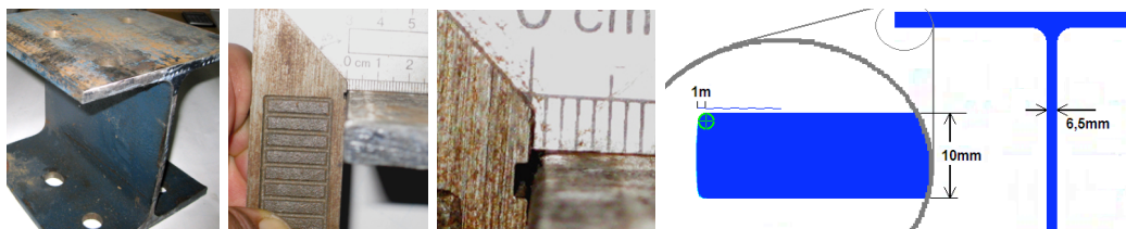
Picture 3: HE A 200, steel rolled beam with a flange radius ( r = 1\text{mm} ).
